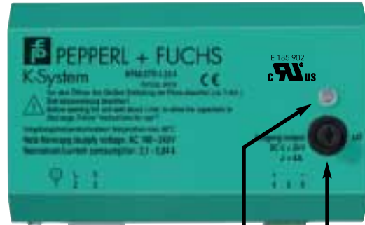
LED GREEN INDICATES OUTPUT VOLTAGE, FLASHING RED INDICATES A FAULT EXISTS FUSE CARRIER
